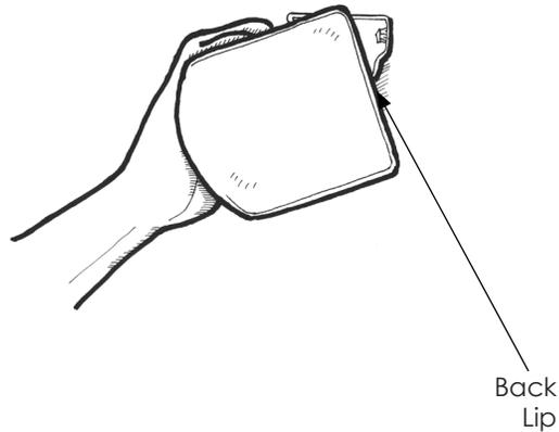
Push the front of the headrail firmly upwards, then roll the headrail up and towards the window opening until it snaps into the brackets.
