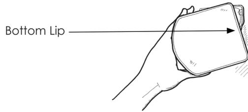
Push the front of the headrail firmly upwards, then roll the headrail up and towards the window opening until it snaps into the brackets.
