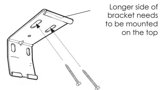
Install the two outside brackets first, no further than 2" in from each end of the headrail.
