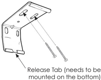
Install the two outside brackets first, no further than 2" in from each end of the headrail.
