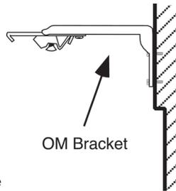
Step 2: Attach an end cap on one end of the track. Install the track into the brackets and tighten the screw.
