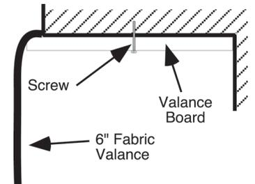
Step 2: Attach the IM brackets to the underside of the valance board. It should be positioned so that the rail will be in the center of the board. DO NOT tighten the screw all the way.
