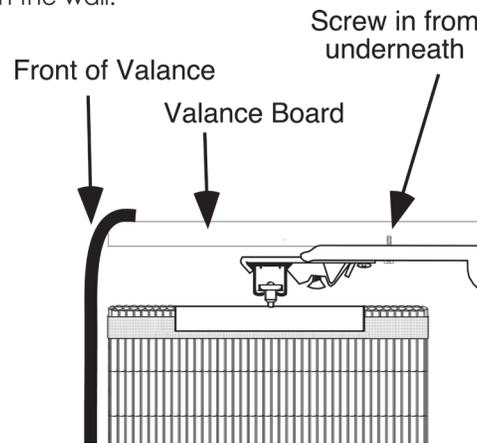
Step 5: Use a 5/8" self tapping screw at each bracket, up from underneath into the headboard of the valance.
